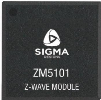
The ZM5101 combines a Z-Wave SD3502 SoC (with a built-in microcontroller and Z-Wave RF transceiver), crystal, and passive RF components within a single 8mm x 8mm module. This makes the ZM5101 ideal for
